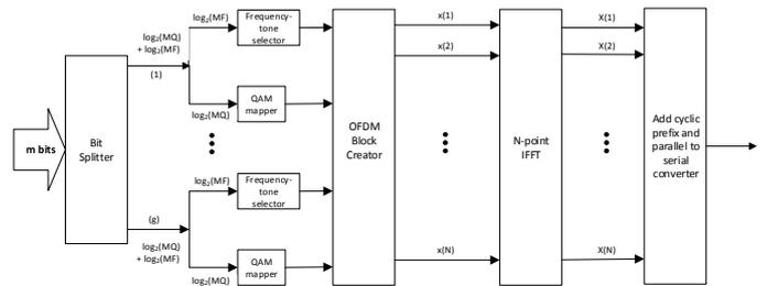
Fig. 2. Block diagram of the FQAM transmitter.
