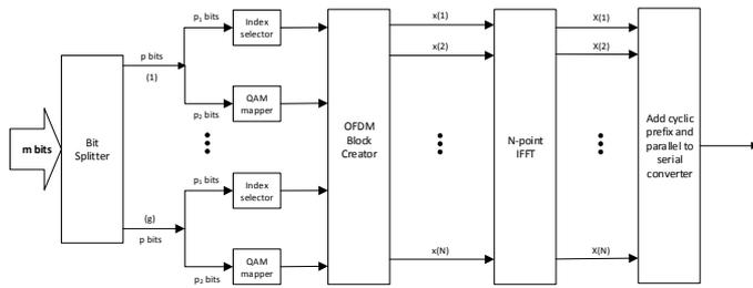
Fig. 1. Block diagram of the OFDM-IM transmitter.
