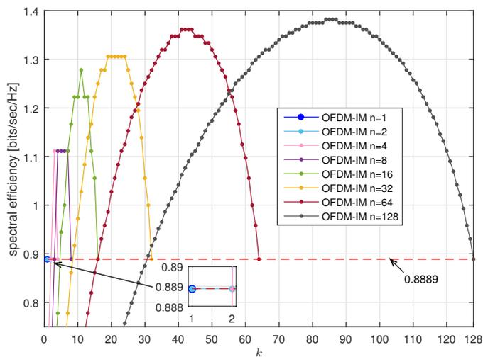
Fig. 5. Spectral efficiency of OFDM-IM.
