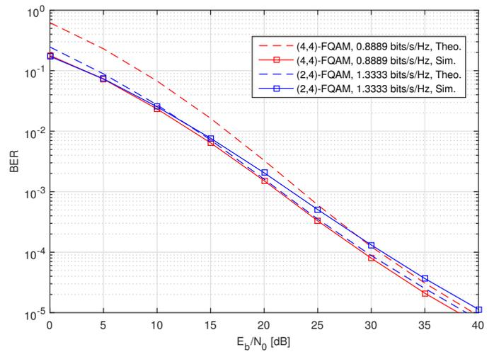
Fig. 4. Theoretical and simulation results for the BER of  $(M_F, M_Q)$ -FQAM.
