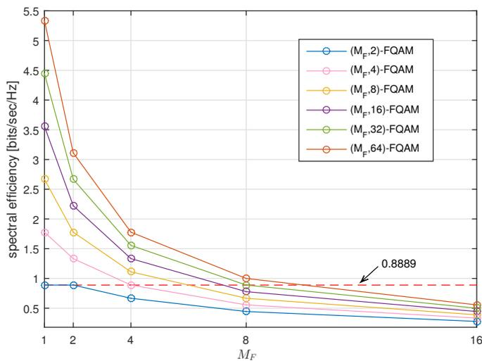
Fig. 6. Spectral efficiency of  $(M_F, M_Q)$ -FQAM.
