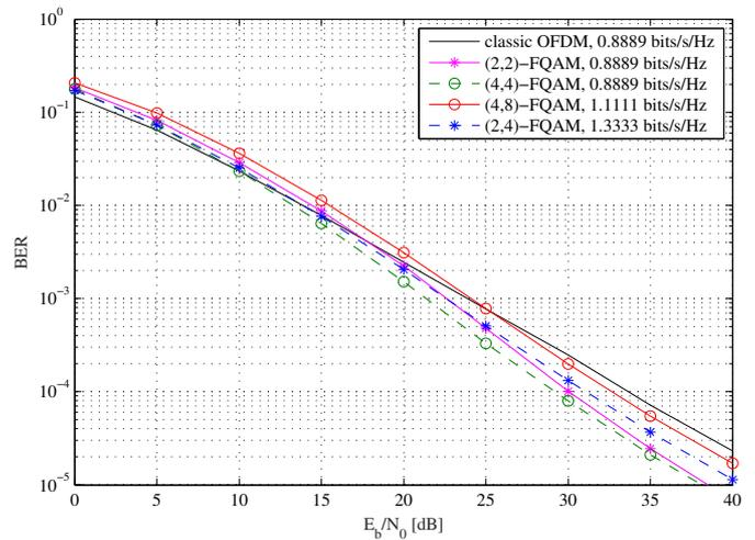
Fig. 8. BER performance of  $(M_F, M_Q)$ -FQAM.
