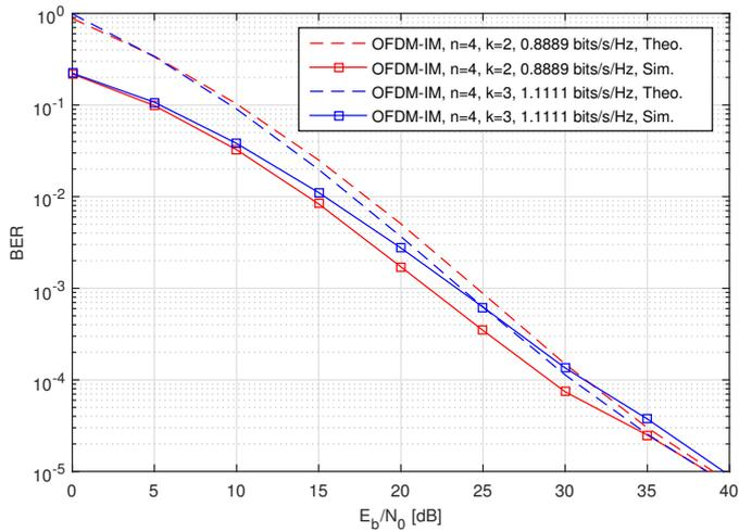
Fig. 3. Theoretical and simulation results for the BER of OFDM-IM.
