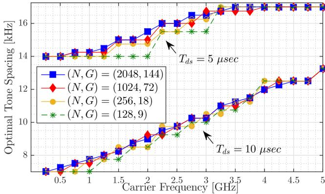
Fig. 2.  $\Delta f_{\text{opt}}$  versus  $f_c$  in OFDM-IM with  $(\nu, m) = (16, 11)$ .
