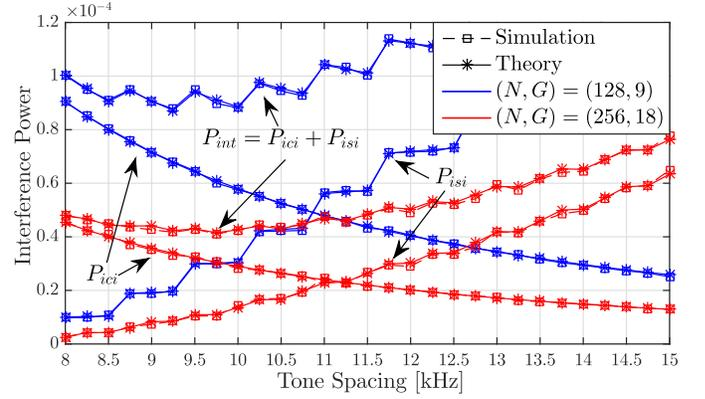
Fig. 1.  $P_{\text{ici}}$ ,  $P_{\text{isi}}$ ,  $P_{\text{int}}$  versus  $\Delta f$  in OFDM-IM with  $(v, m) = (4, 3)$ .
