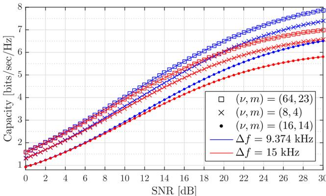
Fig. 4. Capacity versus SNR in OFDM-IM with  $(N, G) = (128, 9)$ , at  $\eta = 1.168$  bps/Hz. The SNR is defined here as  $P_t/(N\sigma_s^2)$ .
